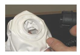
Insert the slotted end of the breathing tube into the hole in the back of the hood. Push the tube until it snaps into place.
