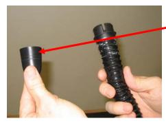
Each PAPR air unit comes with a bullet-shaped pressure check device. Place your thumb and index finger around the slots at the end of the tube so that you force the air through the top of the tube (and prevent air from leaking out the slots themselves). While holding the tube upright, place the pressure check device in the breathing tube.
