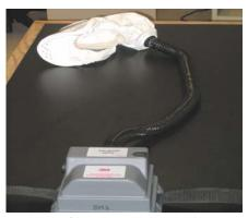
One end of the breathing tube is now connected to the hood; the other end is connected to the air unit.
