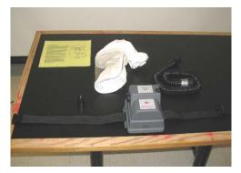
Conduct a pre-use inspection examining all parts of the PAPR for potential damage - breathing tube, hood, air filter unit, and air flow indicator.
