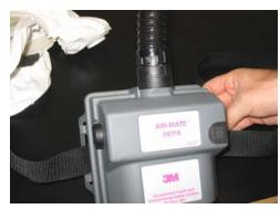
Turn the unit ON by pressing the black plastic button located on the upper righthand side of the air filter unit (this same button is pressed to turn the unit off).
