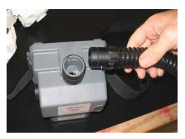
Connect breathing tube to air filter unit by pushing the end of the tube that contains metal clips into the hole in the air filter unit. Twist the tube to secure it to the air filter unit.
