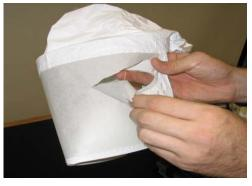
Remove the protective paper from the front of the hood. (Note: Hoods can be reused after cleaning with Virex.)
