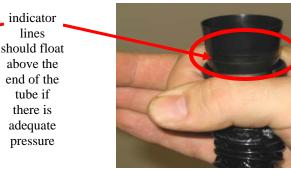
The device should "float" the indicator lines above the end of the tube if the air pressure is adequate. (If it does not, do NOT use the air filter unit. Remove the unit from service and contact SMS at 4-4427.) After the pressure check is complete, remove the pressure check device and turn the unit OFF.
